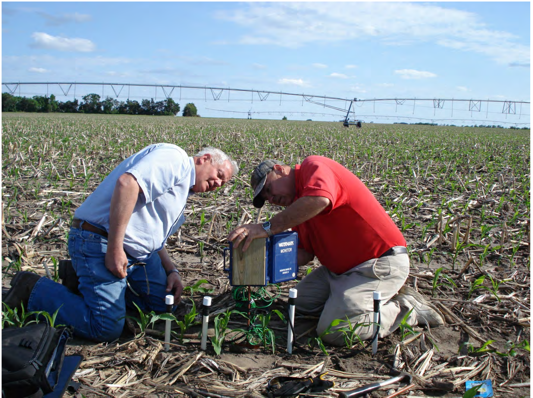
Datalogger programing and sensor installation demonstration
